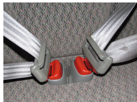
B. Adjacent Buckles: Two side-by-side buckles that could be mistakenly released when two CRs are installed next to each other in a tight space.
