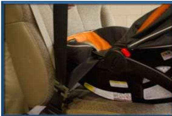
5. Place the belt-shortening clip near the retractor as noted in the vehicle owner's manual.
