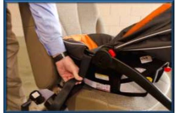
3. Pull on belt to gather the excess webbing to be locked off or shortened near the retractor side.
