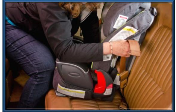
3. Place your hand in the car seat to apply pressure and tighten the seat belt by pulling out the excess slack.
