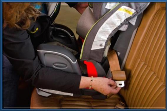
1. Route the vehicle seat belt through the correct car seat belt path.
