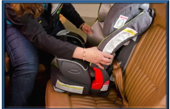
5. Test for a tight installation of the car seat.
