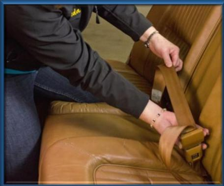
4. Notice the tilt and how the seat belt moves freely. It will hold the webbing locked when **NOT** tilted.
