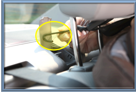
Routing tether straps in vehicles with head restraints
