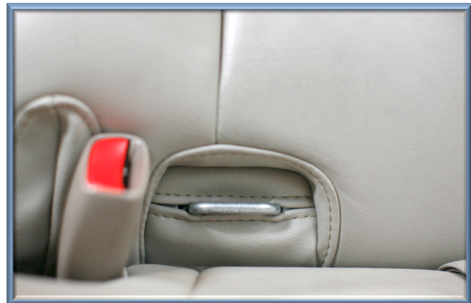
Visible anchor position
