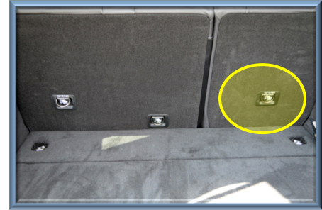
Tether anchor on seat back accessed through rear cargo area
