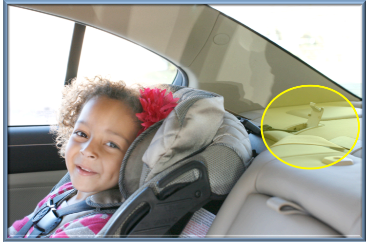
Car seat held in place by tether
