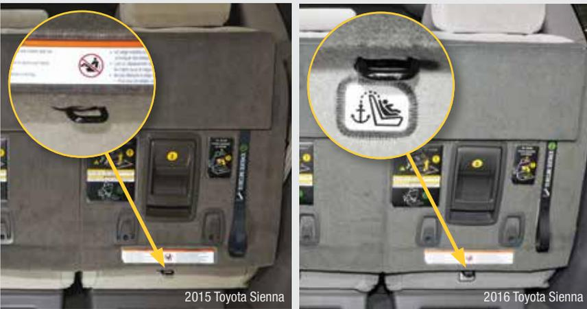
The Toyota Sienna's anchors are at the very bottom of the seatback, near a lot of potentially confusing hardware. In the 2015 model (left), the problem was compounded by the lack of a clear label. In the 2016 Sienna (right), the tether anchors are in the same spot, but a new label makes them more obvious.
