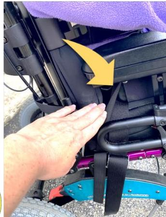
Ample openings for occupant restraint system
