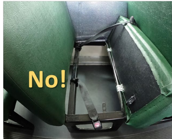
Seat belt knotted around the bus frame
