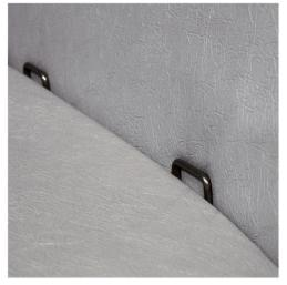
Since 2003, school buses with a GVWR of 10,000 lbs. or less must have a set of lower anchors for two of the bus's seating positions.
